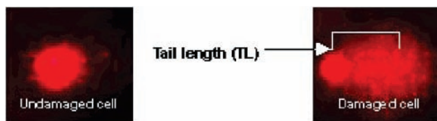
TL = tail length %DNA = DNA of tail given as a percentage Figure 1. Under a fluorescence microscope, the cometlike images resulting from the extension of DNA were scored as a reflection of the single-strand breaks. The tail moment was defined as follows: TM = TL × % DNA.
